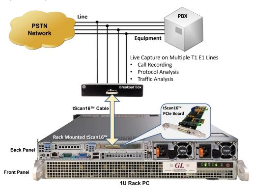
tScan16™ T1 E1 analyzers supports both 32-bit and 64-bit applications. 64-bit support improves the performance of the associated protocol analyzers such as ISDN, ISUP, GSM and allow users to monitor **hundreds to thousands of signaling links** simultaneously and continuously. Also, provides improved processing and response time for **Statistics, Call Data Records, Search,** and other such functions.
