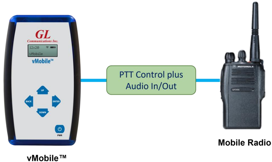
Figure 2: vMobile™ connected to a Push-To-Talk radio.
