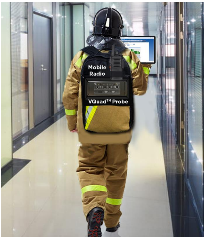
Figure 8: The user tests voice quality while walking in a building by simply using the VQuad™ Probe to connect to the radio and controlling the Indoor Tracking System from a tablet.
