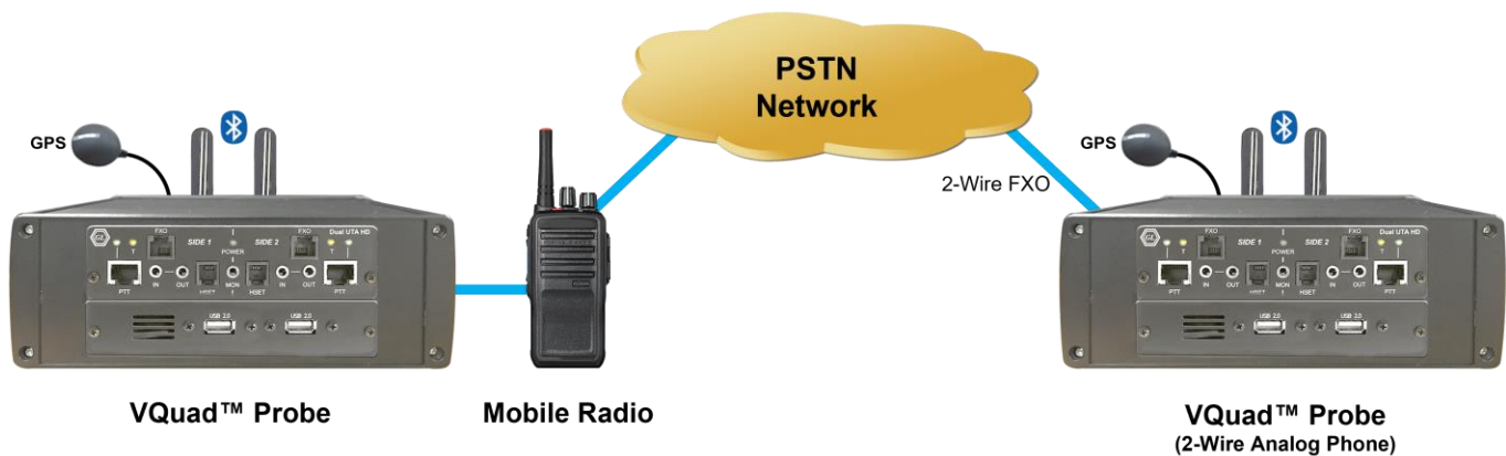
Figure 10: Testing the communication between a mobile radio and the PSTN.
